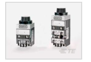
Type of Control: **Knob** Time Delay Relay Input Voltage: **120 – 110 VAC** Timing Range (Off-Time): **1.5 – 15 seconds** Time Delay Relay Contact Current Rating: **10A@240VAC A** Mode of Operation: **Off-Delay**
